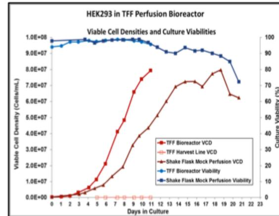
**Figure 3.** VHU Perfusion compared to shake flask centrifugation. Viable cell density using VHU (red circles) versus shake flask mock perfusion (red triangles)
