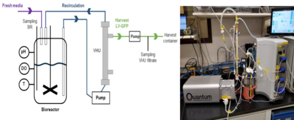
**Figure 1** The VHU™ Perfusion Bioreactor.
