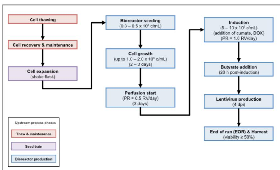
**Figure 2.** VHU™ Perfusion Process using a Stable Producer Cell Line
