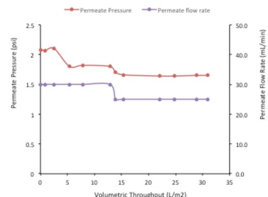
**Figure 5.** Downstream Processing. LV Harvesting: Feed Flowrate: 3L/min; Permeate: 30mL/min; Clarified volume: 1.86 L; Functional titer: 7.58E+06 TU/mL
